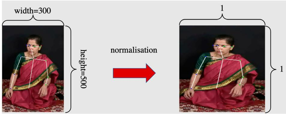
**Figure 2.** Directly normalising the absolute coordinates to  $[0, 1]$  will distort the skeleton and amplify the horizontal movement with respect to the vertical.
