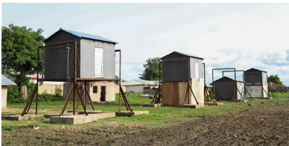
Fig. 1 Experimental huts. From left to right, raised hut without walls below the hut, raised hut with solid wooden walls underneath, hut at ground level (control), raised hut with air-permeable walls underneath. Stairs are shown on the rear face of the second hut from the left only (although in practise all elevated huts had stairs)
