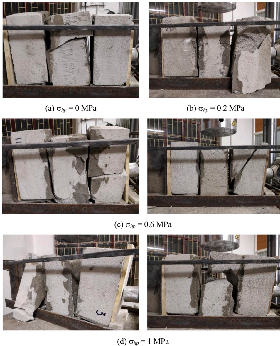
Fig. 14. Failure pattern of AAC masonry triplets at load rate 10 mm/min.
