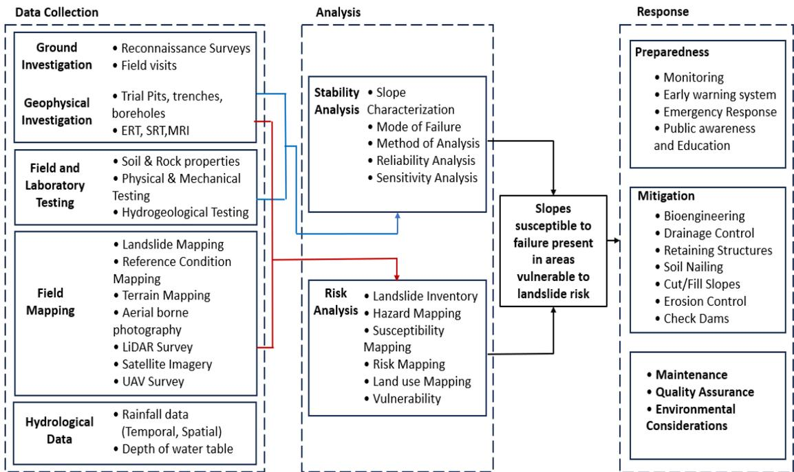
Fig. 9 Proposed road map for landslide analysis and response (ERT: Electrical Resistivity Tomography, SRT: Seismic Refraction Tomography, MRI: Magnetic Resonance Imaging, LiDAR: Light Detection and Ranging, UAV: Unmanned Aerial Vehicle)
