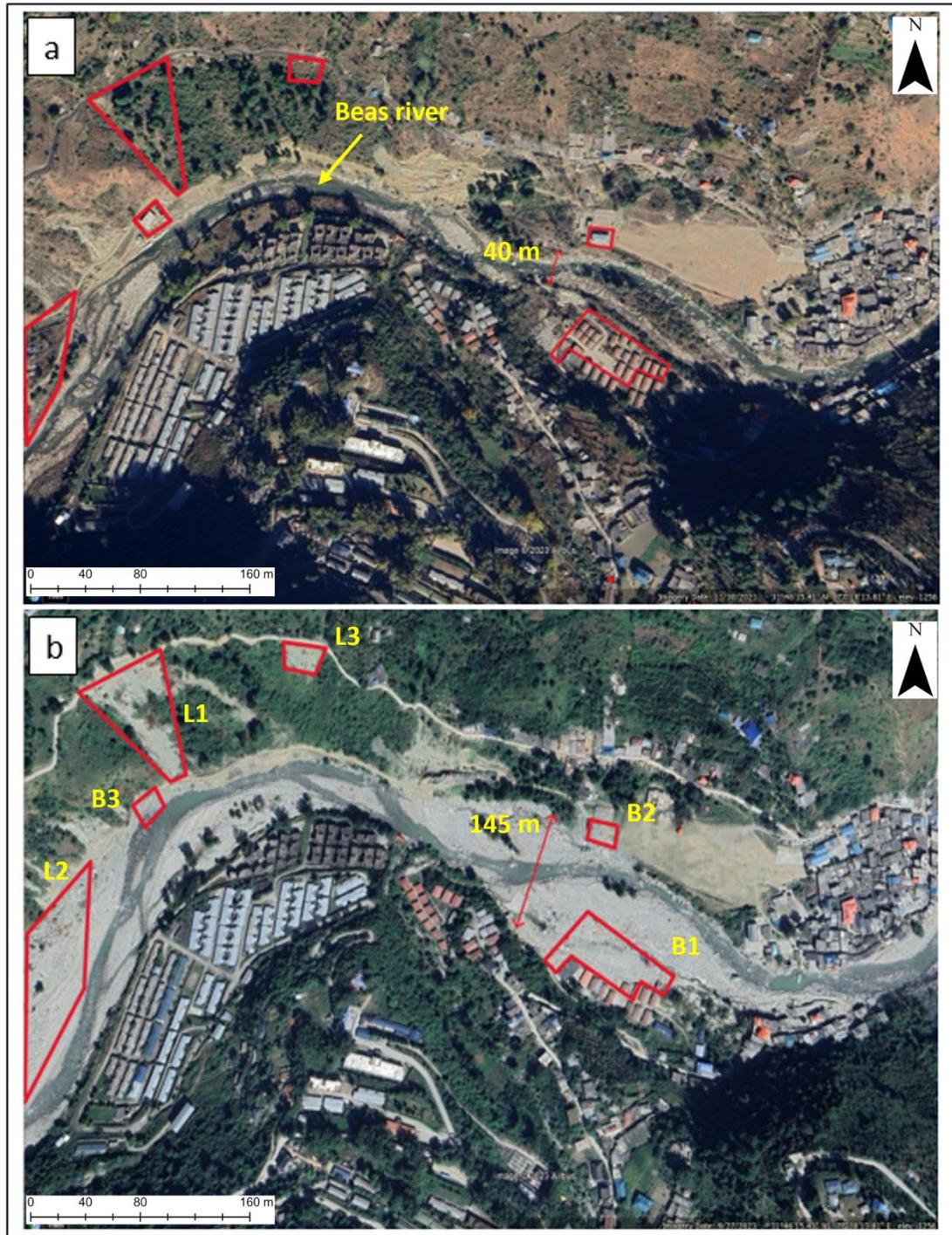
Fig. 8 Satellite images of Sainj area in district Kullu. **a** Before, **b** After the monsoon event of July 2023. [L1, L2, L3 indicate the landslides and B1, B2, B3 indicate building damages] (Source: Google Earth 2023, <https://earth.google.com>. Retrieved 2 November 2023)
