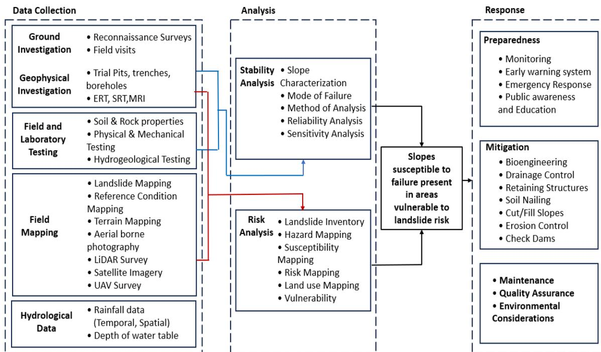
Fig. 9 Proposed road map for landslide analysis and response (ERT: Electrical Resistivity Tomography, SRT: Seismic Refraction Tomography, MRI: Magnetic Resonance Imaging, LiDAR: Light Detection and Ranging, UAV: Unmanned Aerial Vehicle)
