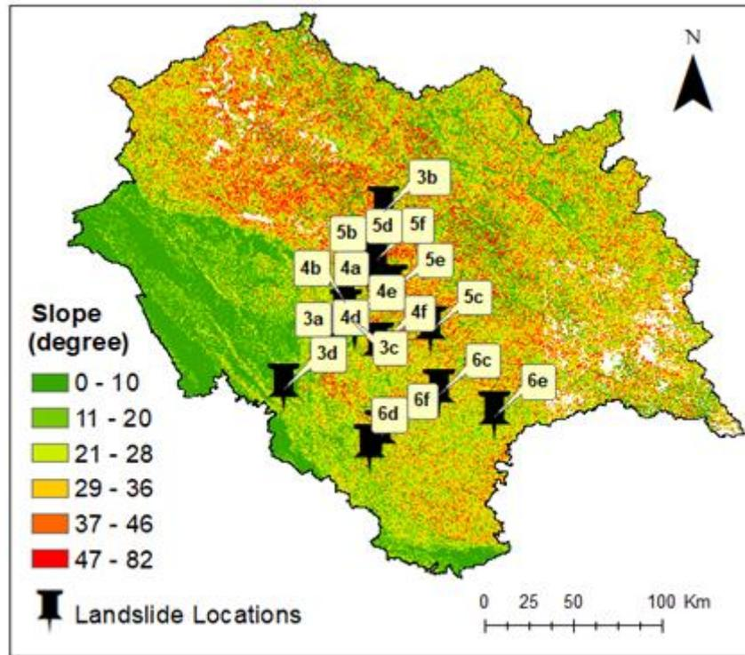
Fig.7 Location of landslides shown in Fig 3,4,5 and 6 compared to slope map (30×30 meters) of Himachal Pradesh (source: Earth Explorer 2023, <https://earthexplorer.usgs.gov/>)
