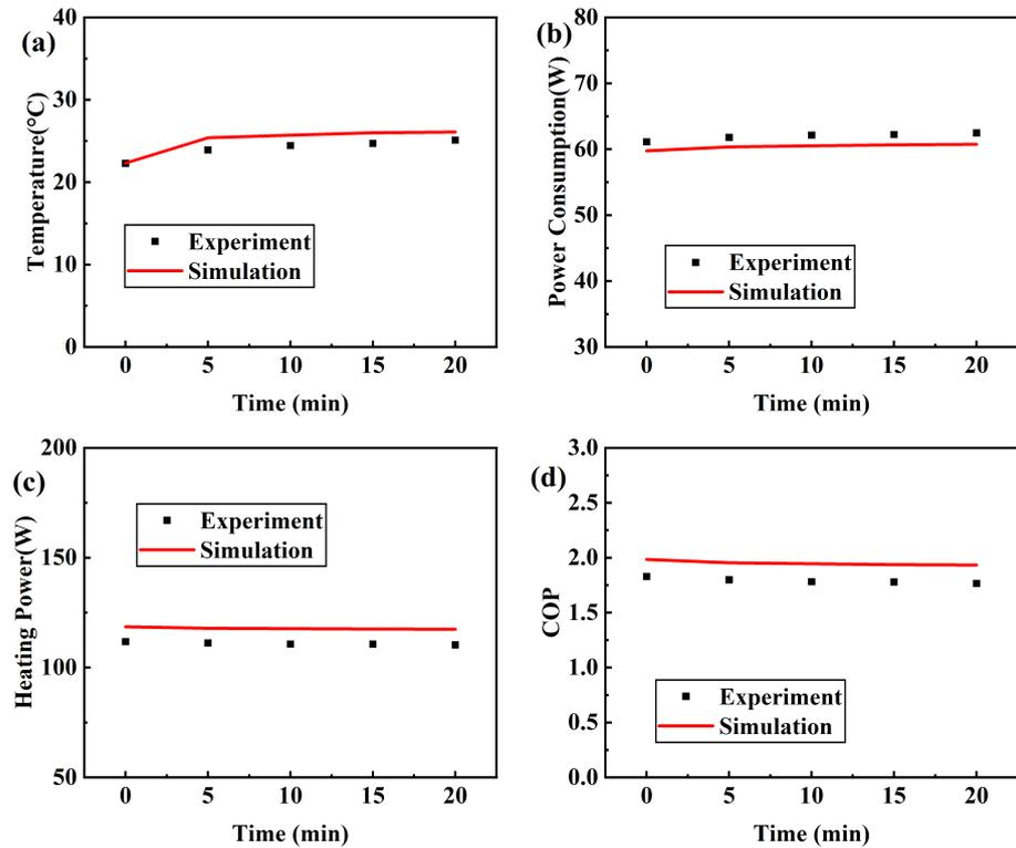
Figure 7. (a) The temperature inside the testing box and the TeHP unit's (b) power consumption, (c) heating power, and (d) COP versus time during Test 3.
