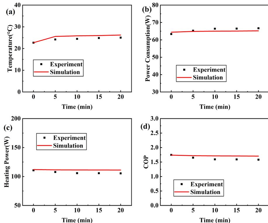
**Figure 4.** (a) The temperature inside the testing box and the TeHP unit's (b) power consumption, (c) heating power, and (d) COP versus time during Test 0.
