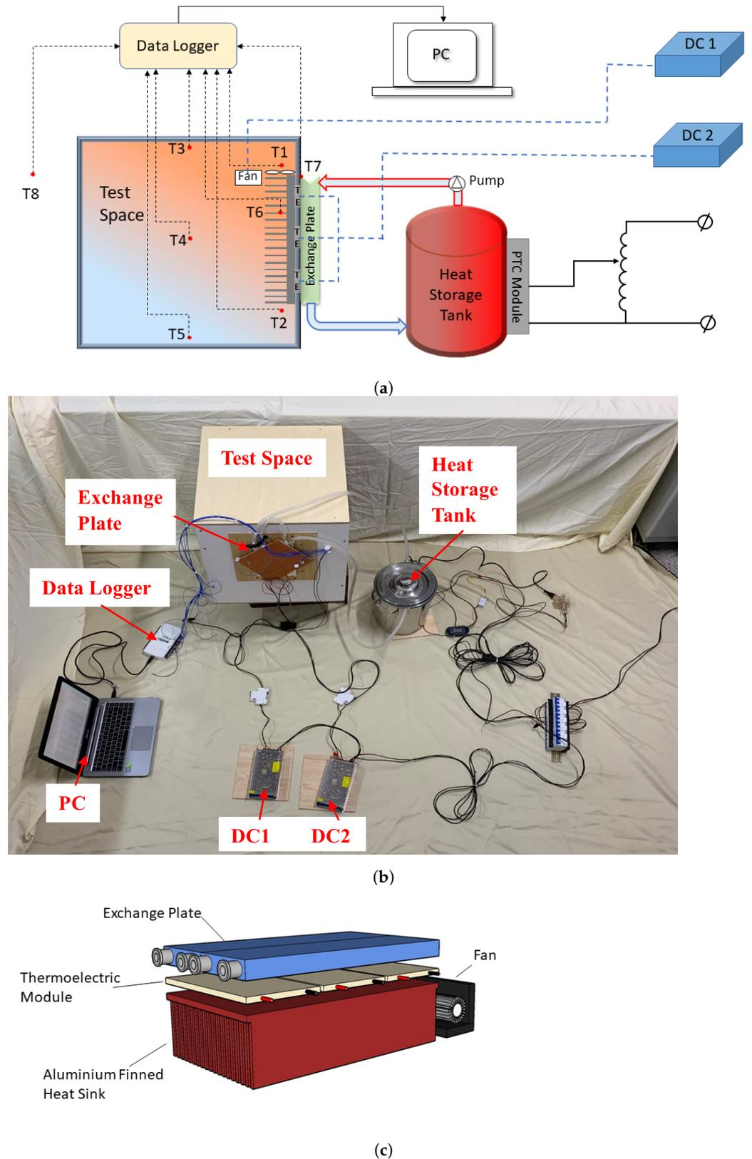
**Figure 1.** (a) Schematic diagram of the experimental apparatus, (b) photograph of the experimental apparatus, and (c) structure of the TE module.
