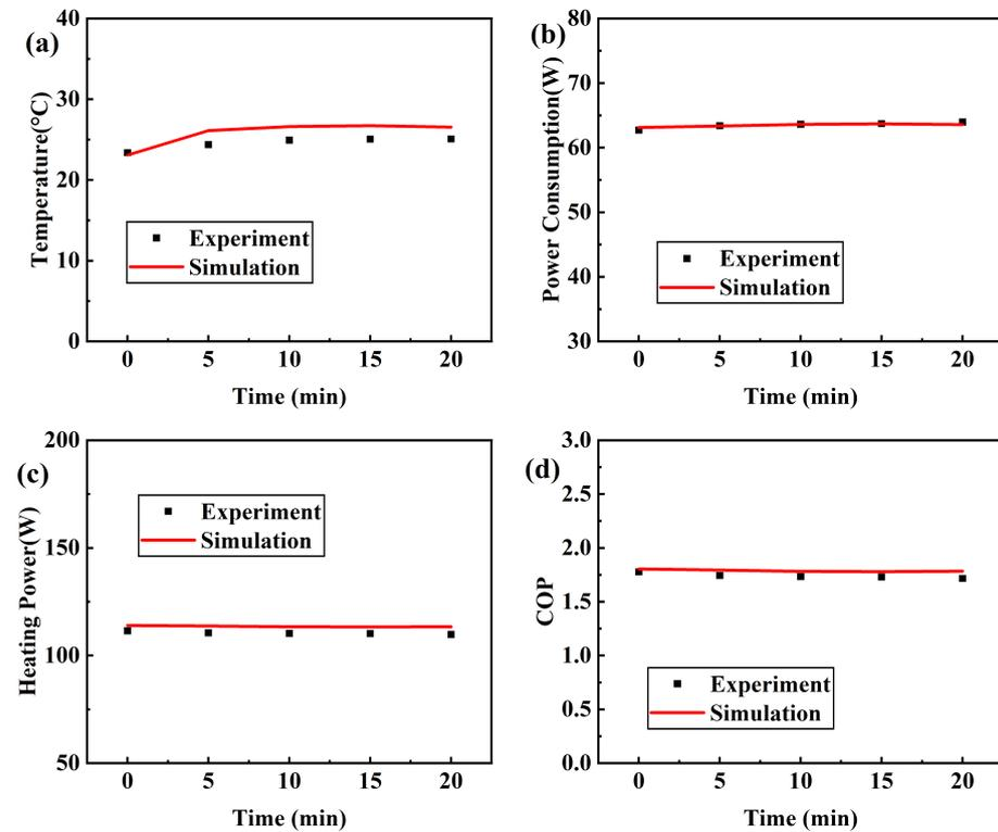
**Figure 5.** (a) The temperature inside the testing box and the TeHP unit's (b) power consumption, (c) heating power, and (d) COP versus time during Test 1.
