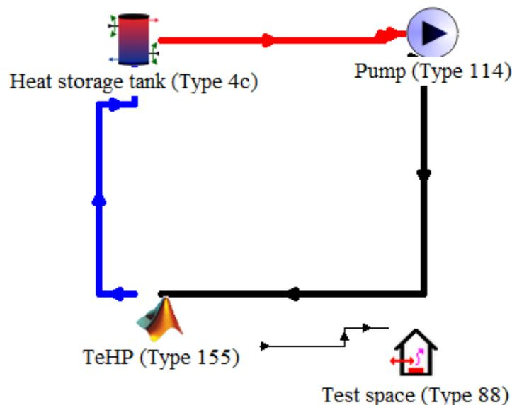
**Figure 3.** Schematic of the TRNSYS project for TeHP simulation.
