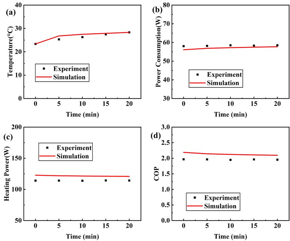
Figure 9. (a) The temperature inside the testing box and the TeHP unit's (b) power consumption, (c) heating power, and (d) COP versus time during Test 5.
