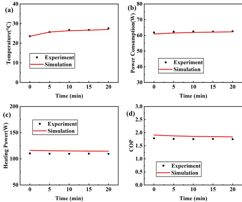
Figure 6. (a) The temperature inside the testing box and the TeHP unit's (b) power consumption, (c) heating power, and (d) COP versus time during Test 2.
