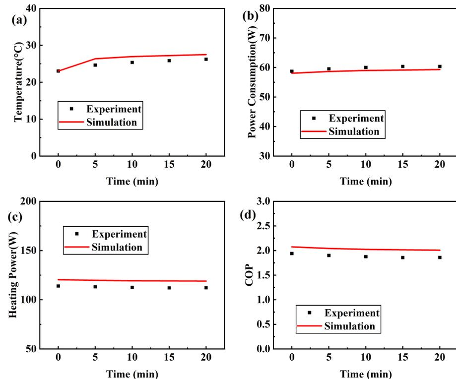
**Figure 8.** (a) The temperature inside the testing box and the TeHP unit's (b) power consumption, (c) heating power, and (d) COP versus time during Test 4.
