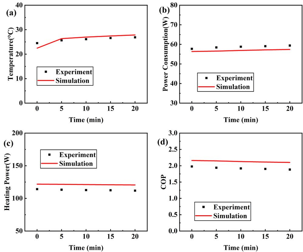
Figure 10. (a) The temperature inside the testing box and the TeHP unit's (b) power consumption, (c) heating power, and (d) COP versus time during Test 6.
