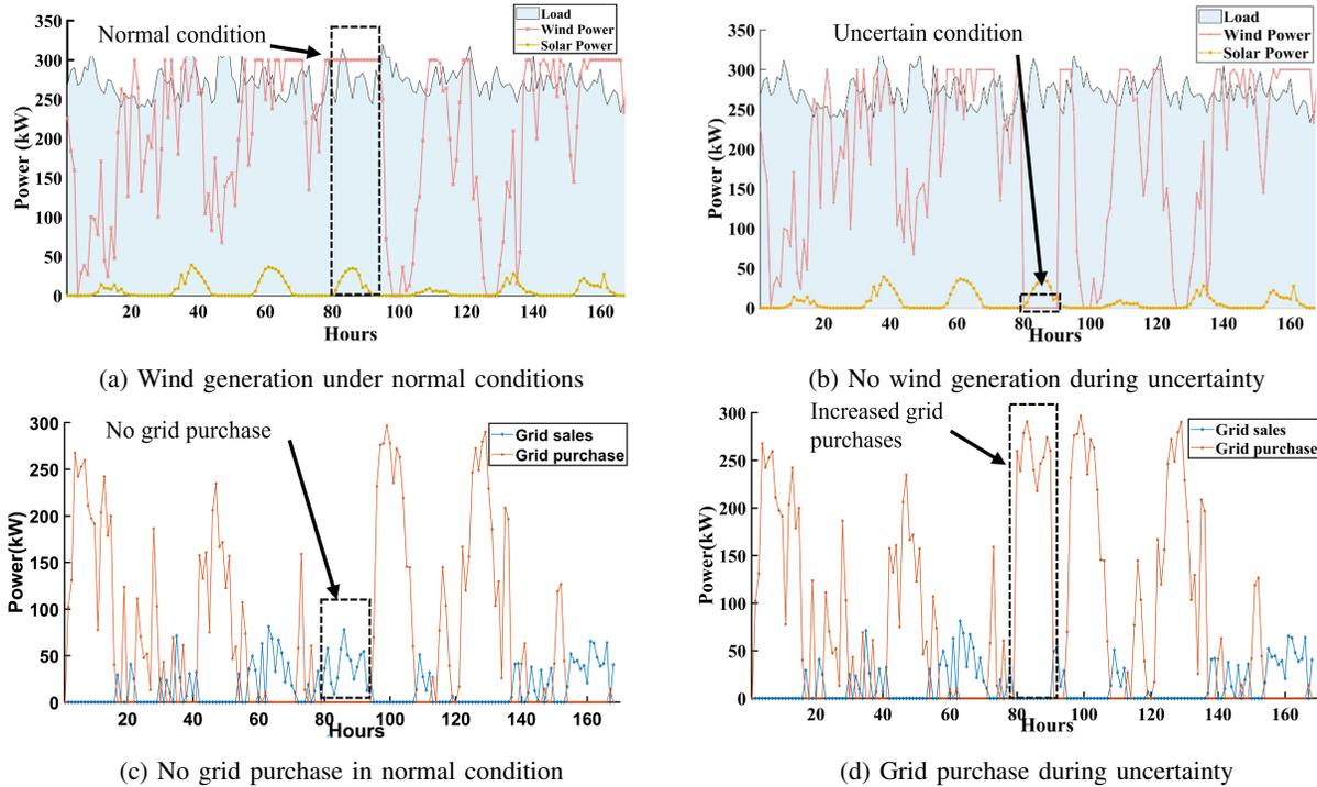
Fig. 6: Energy profiles under different conditions
