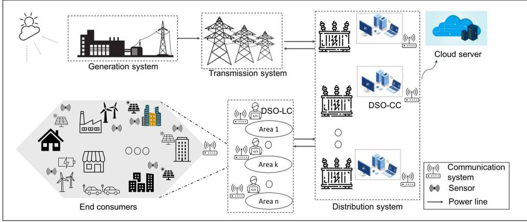
Fig. 1: Power system model with DERs integrated distribution network
