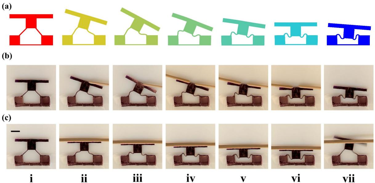
Figure 10. Experimental validation of the MEP from the proposed numerical framework. (a) The shapes of 7 images along the MEP. The red and blue colors denote the stress-free and self-stressed states, respectively. (b) The successful shape transition in the experiment following the MEP. (c) Under a pure compression in experiment, the bistable unit bounces back to the stress-free shape once the constraint is removed. The scale bar is 10 mm.
