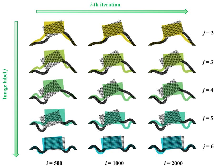
Figure 9. Comparison between the NEB results in the introduced numerical framework (unfilled shapes) and the NEB results that are initiated with a linear interpolation between two stable states (colored shapes). In both cases, the image number is 7 and the spring stiffness  $k_{NEB} = 4 \times 10^{-3}$  N/mm.
