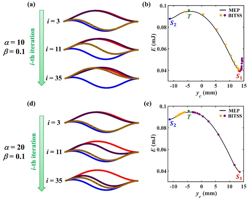
Figure 6. The transition path for a buckled beam with  $\varepsilon_c = 5\%$ ,  $\phi_1 = 17^\circ$ ,  $\phi_2 = 0^\circ$ . The shapes and energy of the two images during iterations in the BITSS method are shown in (a) and (b) when  $\alpha = 10$ ,  $\beta = 0.1$ , in
