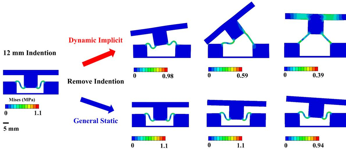
Figure 11. Comparison between the dynamic and static simulations. After removal of 12 mm indentation, the bistable unit can snap back to  $S_1$  under dynamic analysis (top row) or converge to  $S_2$  nearby under general static analysis (bottom row). The scale bar is 5 mm.
