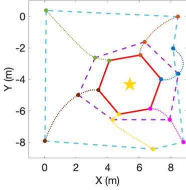
Fig. 2. Trajectories of the six robots with a fixed centroid (yellow star).
