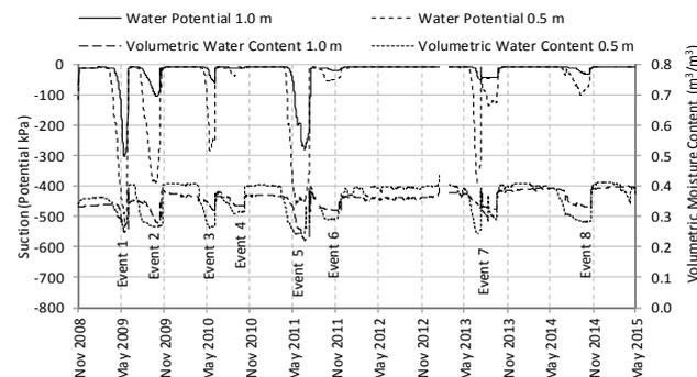
Figure 3. Volumetric water content and soil-water potential records from position MP1 at 0.5 and 1.0 m depth.
