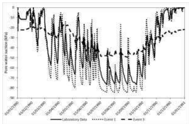
Figure 8. Pore-water suctions at the slope toe for the differing soil water retention curves.
