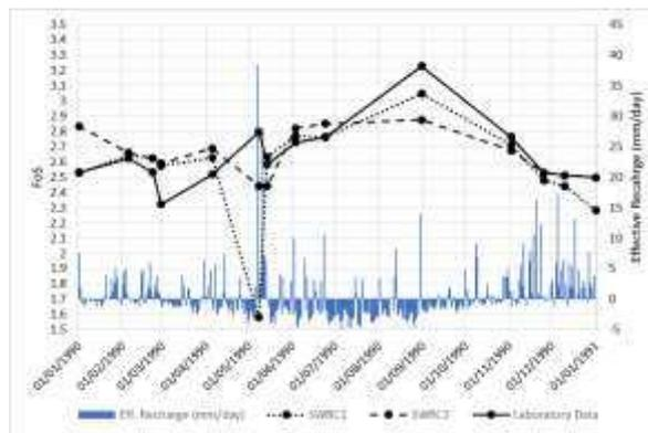
Figure 9. FoS changes within slopes with differing SWRCs.
