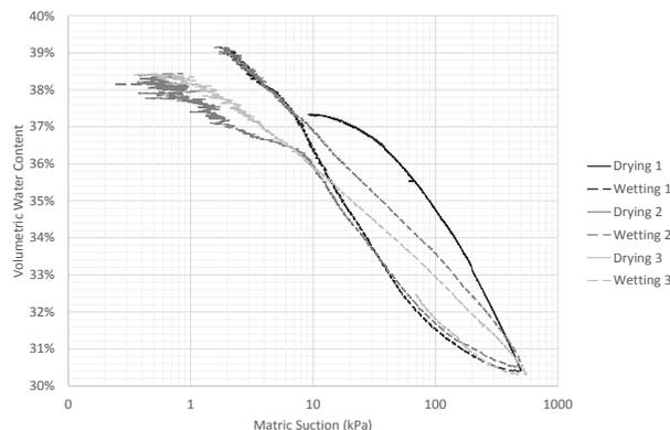
Figure 6. Soil Water Retention Curve Cycling between 0 and 500 kPa
