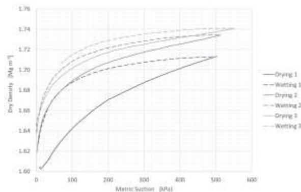
Figure 7. SWRC Dry Density Variation Cycling Between 0 and 500 kPa
