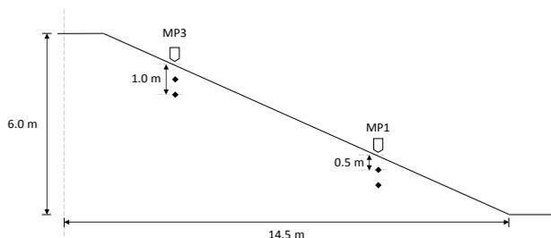
Figure 2. Slope schematic showing layout of sensor pairs.
