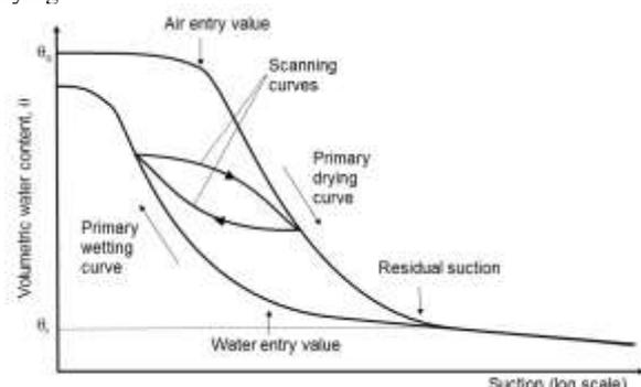
Figure 1. Typical Soil Water Retention Curve (after Toll, 2012)
