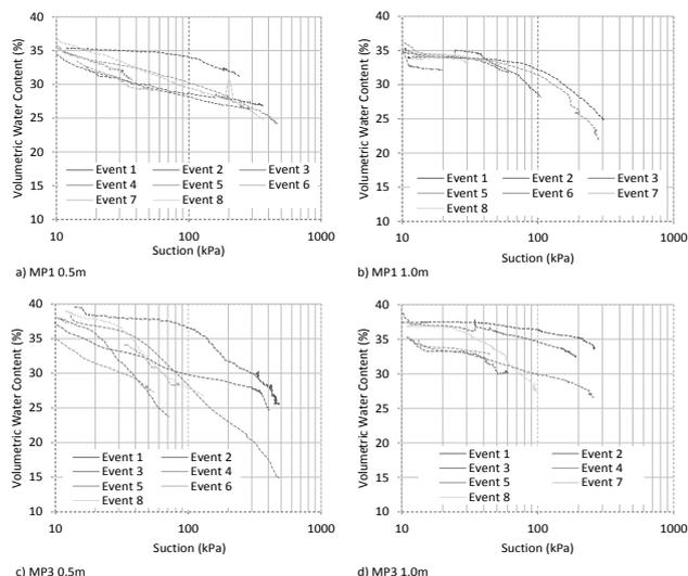
Figure 4. In situ SWRCs as measured at (a-b) slope toe and (c-d) slope shoulder at 0.5 and 1.0 m depth.
