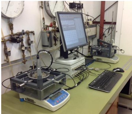
Figure 4. The Durham SWRC equipment, showing the frame sitting on the electronic balance.
