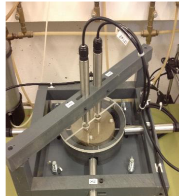
Figure 5. The Durham SWRC equipment, showing the PVC frame with LVDTs to measure volume change.
