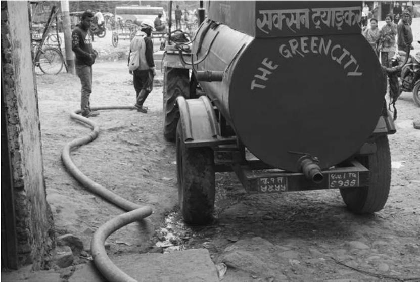
Figure 11. Desludging truck, Nepal. Source Dave Robbins, CC BY-SA 2.0.
