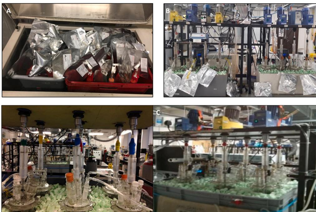
**Fig. 1.** Fermenters employed for the different anaerobic digestion studies with gas and feeding outlets, a) batch mode (500 mL) in an automated stirred incubator system and continuous system (CSABR) b) 1 L and c) 5 L.
