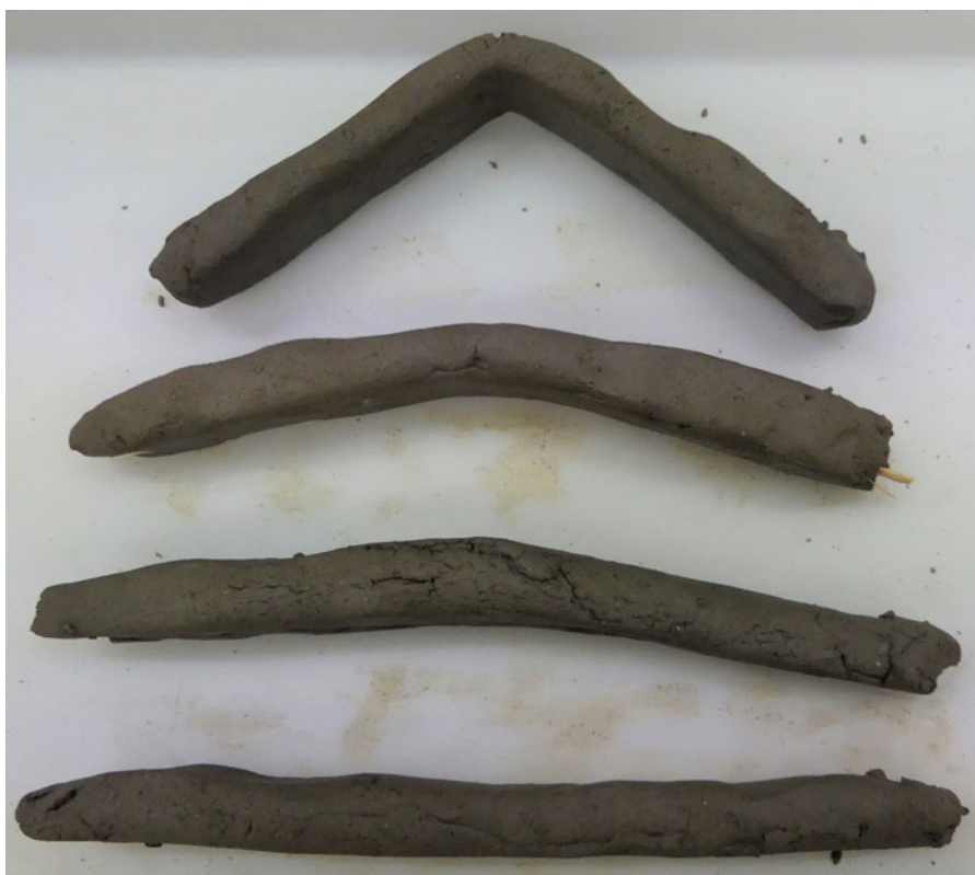
Fig. 8. Experimental tablets showing effects of holding by the middle while wet. From top to bottom: rolled, without straw; rolled, with straw; folded, without straw; folded, with straw. Photo: author.
