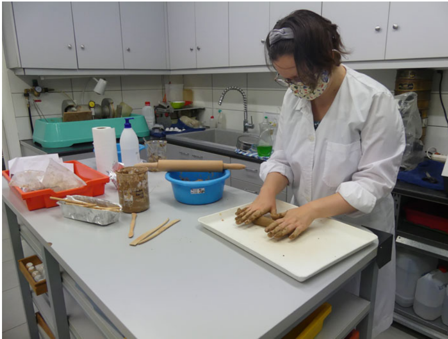
Fig. 2. The author rolling out a cylinder of clay to form a tablet in the Fitch Laboratory. Photo: Evangelia Kiriati.
