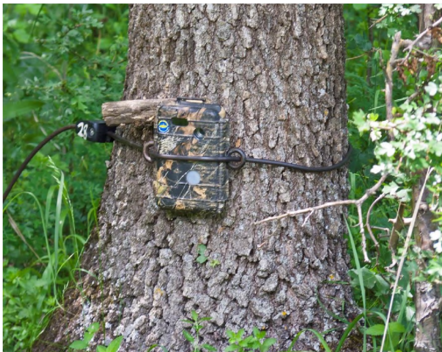
Fig. 2. A camera trap attached to a tree using a security lock. The bit of wood wedged behind the camera is placed to ensure the camera angle is correct with respect to the ground in front.
