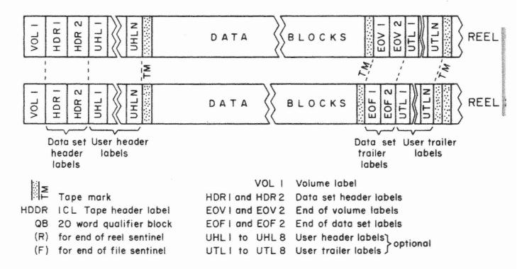
Figure 4. Standard label format for a single data set spanned over two reels
