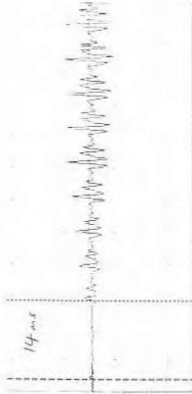
Speech waveform for /h/: left cursor marks release burst, right cursor marks voice onset.
