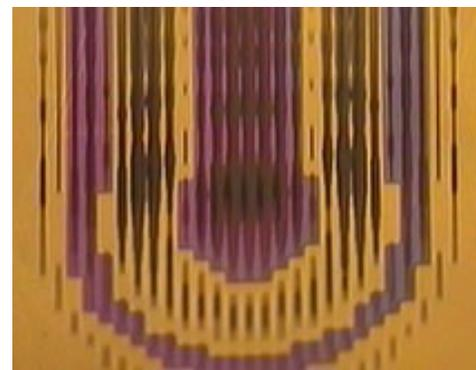
**Figure 14** Binary phase/pseudo greyscale CGH using slits
