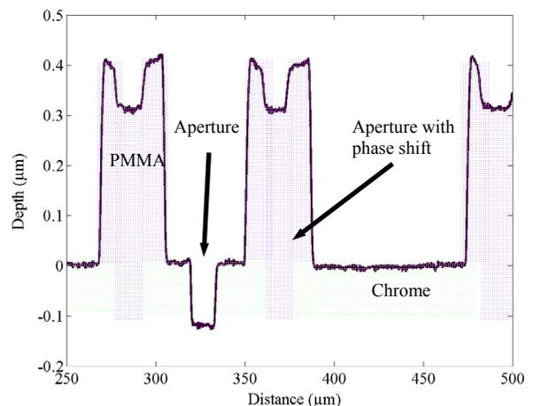
**Figure 10 Surface profile of section of a binary phase/pseudo greyscale amplitude CGH mask**
