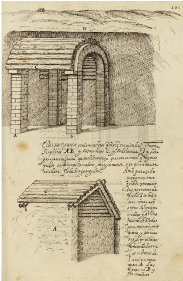
Fig. 6 How to line the tunnel in the 'mine' in the 16th century, according to Lastanosa (1601).
