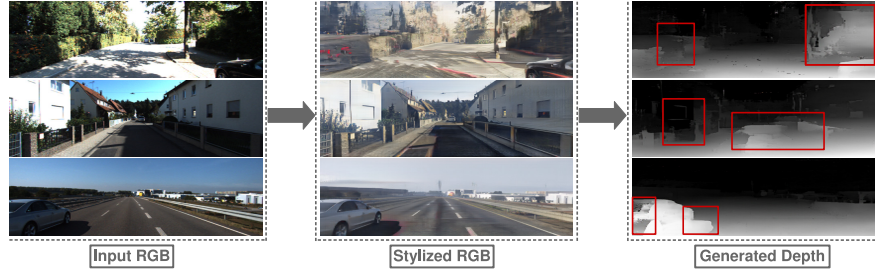
Fig. 7: Examples of failures, mainly due to light saturation and shadows.
