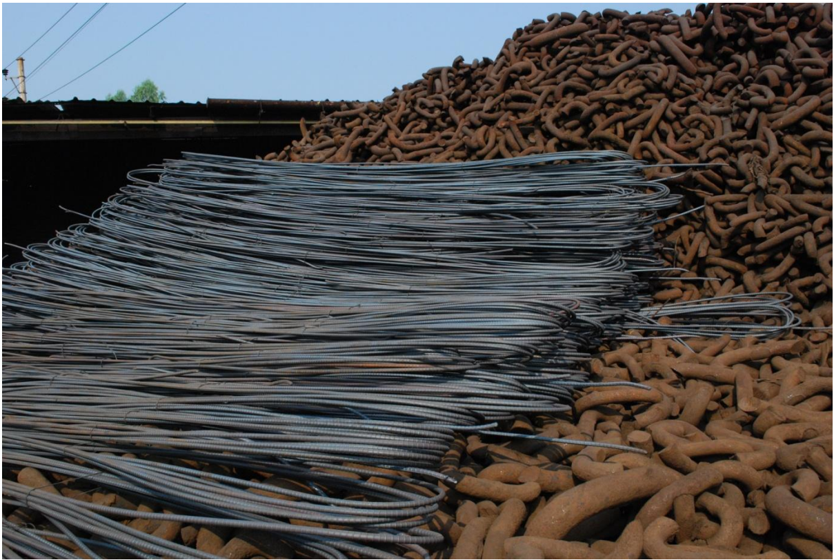
Caption: The afterlives of steel: ships cable becomes reinforcing rod for buildings
