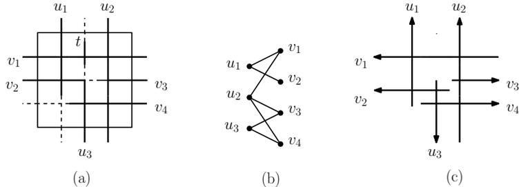
**Fig. 1.** (a) A nano-wire crossbar with disconnected wire defects, (b) the bipartite graph modeling this crossbar, and (c) a 4-DORG representation of this graph. Note that vertex  $t$  is not present, since the corresponding wire is not connected to the crossbar boundary, hence with the remaining circuit.
