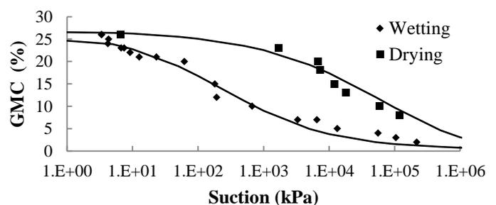
Figure 1. Soil Water Retention Curve. Data points from Shehu (2011).
