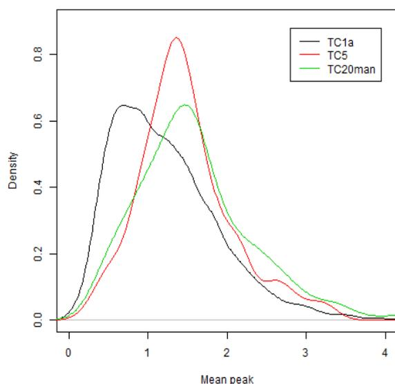
**Figure 5: Figure Peak 2: Distribution of the annual max 4-8pm peak in kW for TC1a, TC5 and TC20(IHD) (solar generation is excluded for solar test cells)**
