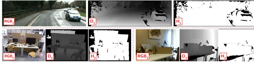
Fig. 1.1: Examples of depth acquired via stereo correspondence (top), structured light device (bottom left) and time-of-flight camera (bottom right). **RGB**: colour image; **D**: depth image; **H**: hole mask indication missing depth values.
