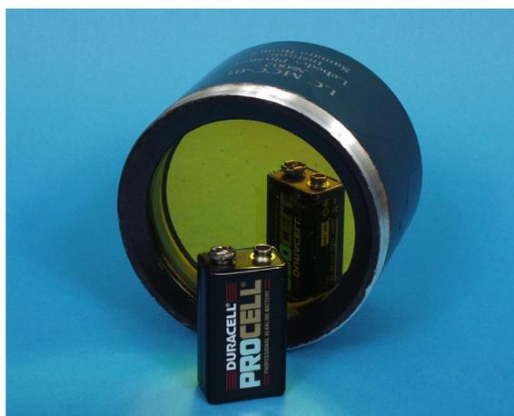
Fig. 15. A larger aperture (70mm) liquid crystal modal wavefront corrector (the battery is shown for scale).
