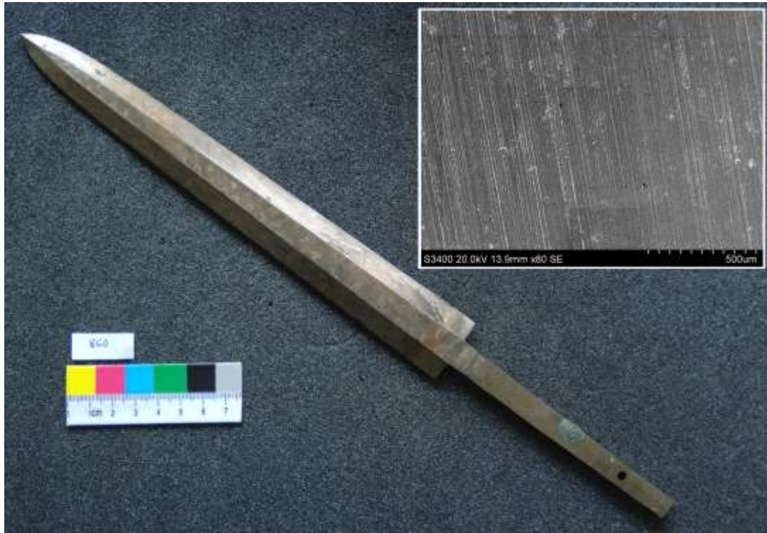
Fig. 5. A bronze lance from the Terracotta Army, with (inset) SEM image of a silicon rubber impression taken on a lance blade, showing the fine polishing marks (original image from 2 ©Imperial Logistics Project).
