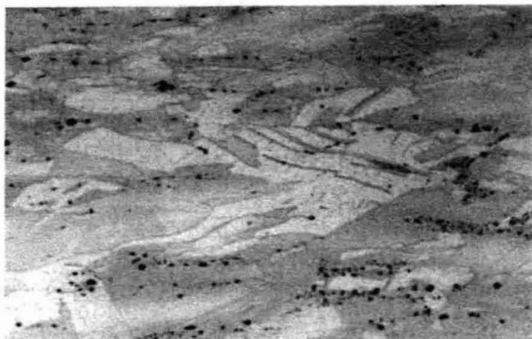
**Figure 9.** 180046. EB II axe (near to blade). Original magnification  $\times 200$ . Etched. Shows copper-copper oxide eutectic which is distorted into lines of 'droplets'. Recrystallised grains and annealing twins are visible. The grains are not equi-axed and the annealing twins also show some distortion. There is no sign, however, of any strain lines.
