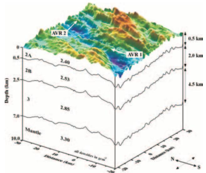
**Figure 7.** Example from the simple crustal model used for the MBA calculation. Layers of constant density and thickness are draped beneath the seafloor topography. The thickness and density of each layer are annotated.
