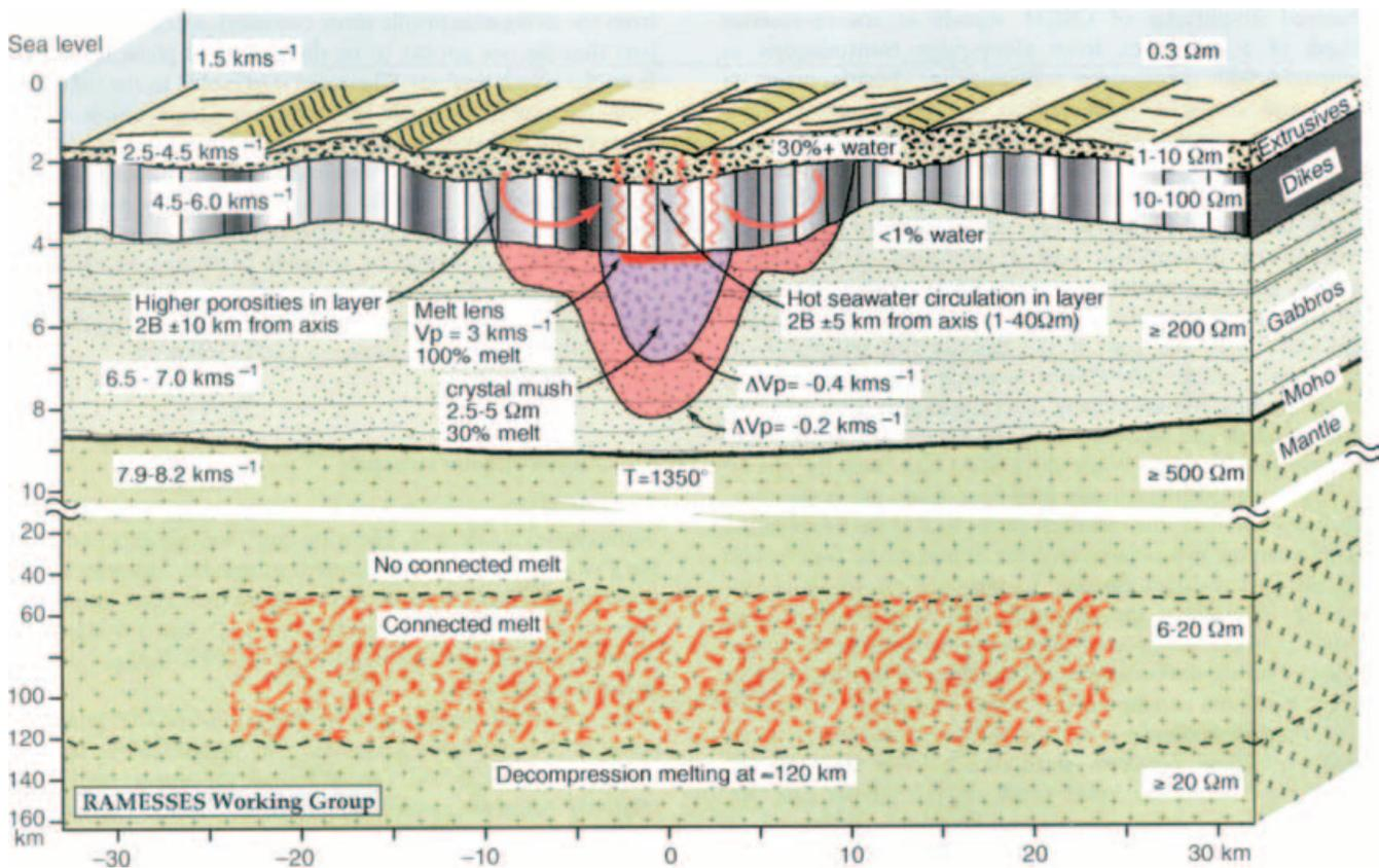
**Figure 1.** Cross-sectional model of the 57°45'N AVR based on a synthesis of the modelling and interpretation of RAMESSES data sets. The analyses of seismic, gravity, electromagnetic and magnetotelluric data suggest that a magma chamber underlies this AVR and that a zone of partial melt extends from ~50 to 100 km depth in the upper mantle. Note that a break in scale occurs at a depth of 10 km below sea level. After Sinha *et al.* (1998).
