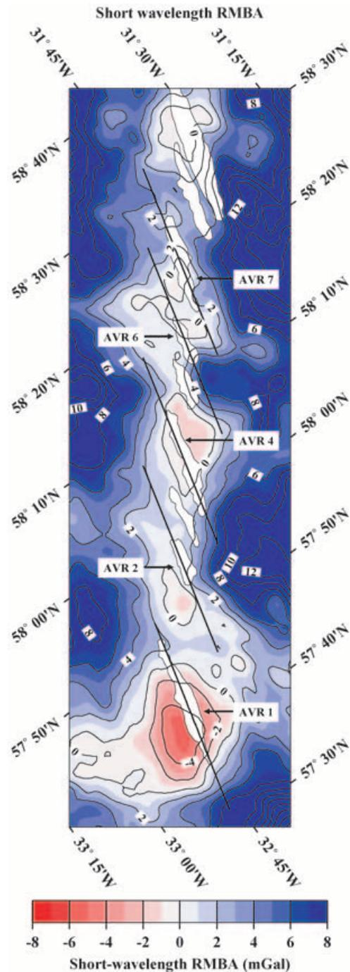
**Figure 10.** RMBA with the linear ‘regional’ trend shown in Fig. 9 removed to highlight AVR-related features. A broad low follows the ridge trend with small ‘bull’s eye’ lows associated with a number of AVRs superimposed. Solid lines show the profiles extracted to model the crustal structure of the selected example AVRs (see Figs 11–15). AVR footprints are superimposed in white for clarity and the chosen example AVRs labelled. Contours are plotted at 2 mGal intervals.
