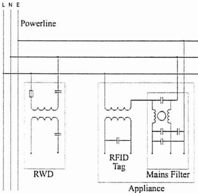
Figure 9: Experimental passive system showing coupling of RFID tag and RWD. Utilisation of a typical appliance mains filter is also shown.
