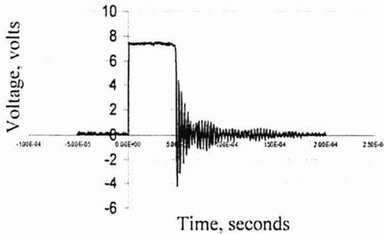
Figure 8: Coupler protection by transient voltage suppressor.
