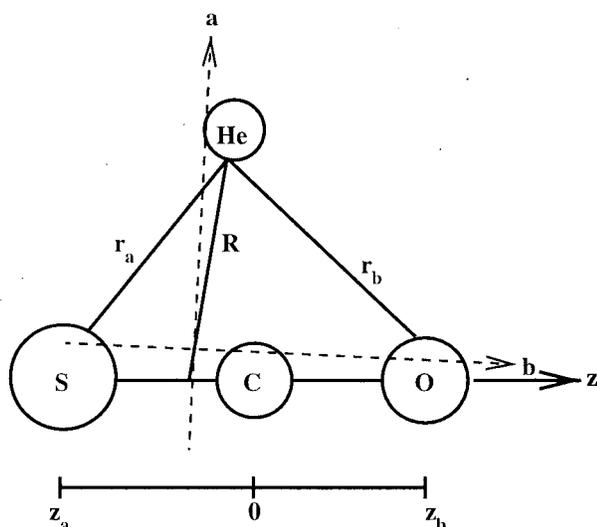
FIG. 1. The He–OCS inertial axes and distances used to define prolate spheroidal coordinates.
