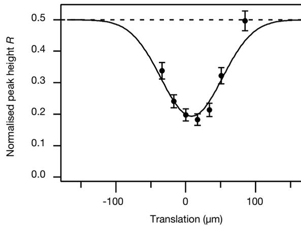
Figure 3: Ratio of the height of the residual peak at zero delay in the beamsplitter configuration to the average height of the peaks in the beam separator configuration, as a function of the relative distance between the two beams, translated parallel to each other. The solid curve is the expected ratio, calculated from the measured beam waist of the two beams. The amplitude and the center of this curve is adjusted to fit the data. The error bars correspond to statistical uncertainties.
