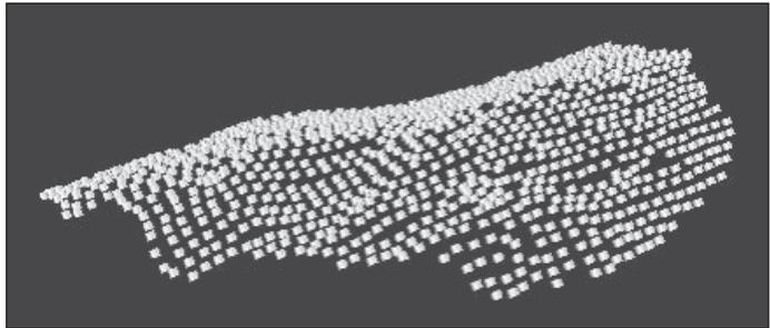
*Figure 7. Marked and referenced targets in Photomodeler.*
