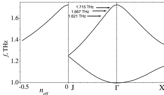
Fig. 2. Band structure [13] of the hexagonal photonic crystal with lattice constant of 200  $\mu\text{m}$  formed by metallic rods of diameter 80  $\mu\text{m}$ . Horizontal arrows indicate the frequencies for which the modelling of the field pattern is shown in Fig. 3.
