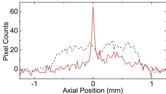
FIG. 3: Column density for a CO<sub>2</sub> laser lattice without the Nd:YAG laser (dashed line), and for a shallower CO<sub>2</sub> laser lattice with the Nd:YAG laser (solid line). The overall ground state light-shift in the overlap region of the shallow combined trap (−27 MHz) is less than the maximum light-shift for the CO<sub>2</sub> laser lattice alone (−36 MHz), but loading into the combined trap is still significantly more efficient. Both profiles are for a molasses detuning of −20 MHz.
