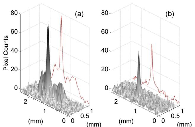
FIG. 2: A surface plot of the column density for cooling laser detunings (a)  $\Delta = 2\pi(-20 \text{ MHz})$  and (b)  $\Delta = 2\pi(+2 \text{ MHz})$ . The on-axis density is shown on the back plane. For blue-detuning (b) only the light-shift engineered region, where the CO<sub>2</sub> and Nd:YAG laser beams overlap, is loaded.
