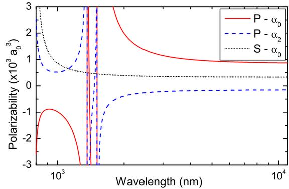
FIG. 4: Calculated polarizabilities of the  $5s$  and  $5p$  states of Rb. For the  $p$  state we show the scalar and tensor polarizabilities,  $\alpha_0 = (\alpha_{xx} + \alpha_{yy} + \alpha_{zz})/3$  and  $\alpha_2 = (\alpha_{xx} - \alpha_{zz})/3$ , respectively. For the  $s$  state,  $\alpha_0 = \alpha_{xx} = \alpha_{yy} = \alpha_{zz}$ .
