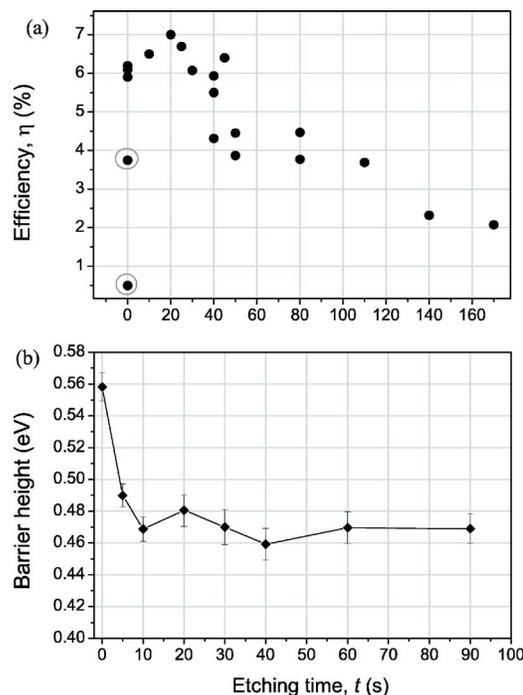
FIG. 6. Dependence on the NP etching time of (a) light conversion efficiency and (b) back-contact barrier height. NP etching reduces the large scatter of efficiencies seen for unetched cells and eliminates low performing contacts (circled points).
