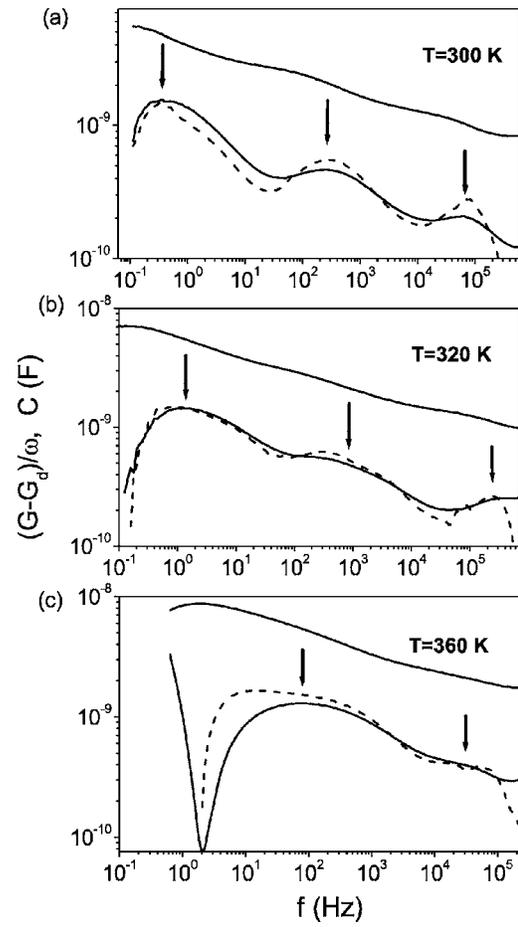
FIG. 1. AS data measured at different temperatures for an unetched sample (sample I). Lower solid lines, frequency dependence of normalized conductance  $(G-G_d)/\omega$ ; upper solid lines, frequency dependence of capacitance  $C$ . The dashed lines correspond to the logarithmic derivative:  $(-\pi/2)dC/d \ln f$ . The arrows indicate the positions of the conductance peaks—they shift with increasing  $T$ .
