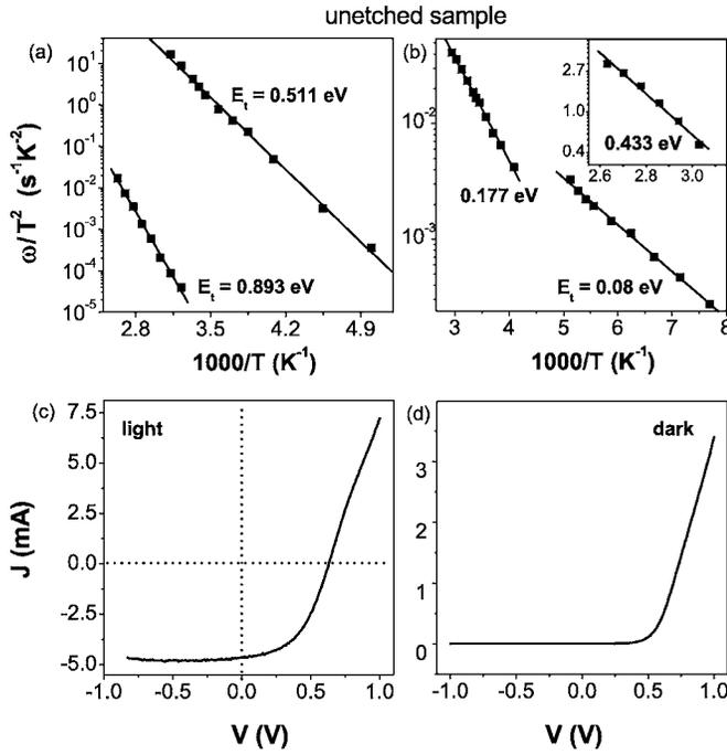
FIG. 2. [(a) and (b)] Arrhenius plot of the normalized conductance peak positions for sample I (unetched). Symbols, experimental data; solid lines, linear fits. [(c) and (d)] light and dark  $I$ - $V$  characteristics of the same sample.
