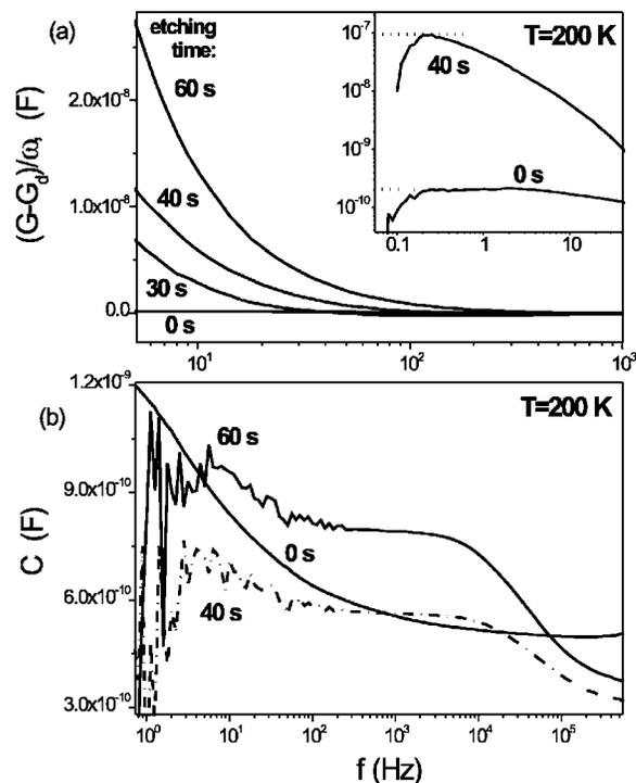
FIG. 5. (a) Normalized conductance in the low-frequency range for samples I, IV, V, and VI (etched for  $t = 0, 30, 40,$  and  $60$  s, respectively). Inset: Zoom-in of the data at  $f < 10$  Hz for samples I and V. (b) Low-frequency capacitance for samples I, V, and VI, demonstrating the drastic change in  $C(f)$  caused by the NP etching at  $f < 100$  Hz. The data in (a) and (b) were obtained at  $T = 200$  K.
