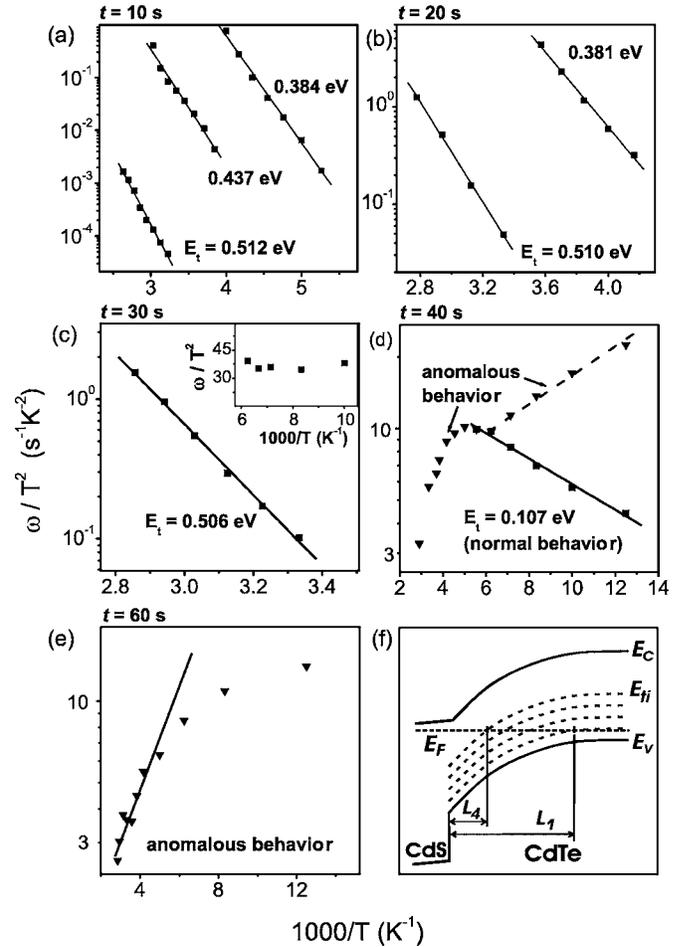
FIG. 4. [(a)–(e)] Arrhenius plots of the peak positions of admittance maxima for five samples (II–VI), etched for different time  $t$  as indicated on the plots. Symbols, experimental data; solid lines, linear fits. (f) Band diagram of  $p$ - $n$  junction in CdS/CdTe solar cell. The dashed lines indicate positions of deep and shallow levels.
