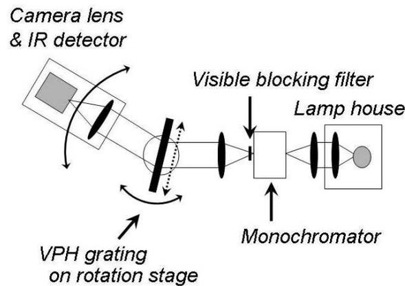
Fig. 2. Schematic view of the test optics configuration.
