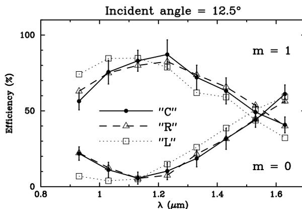
Fig. 4. Diffraction efficiency measured for an incident angle of  $12.5^\circ$ . Throughputs measured at the centre are shown by solid circles (and solid line), and those at the other two positions are indicated by open triangle (and dashed line) and open square (and dotted line). The upper three lines are for the  $m = +1$  order diffracted light and the lower ones are for the 0th order light.
