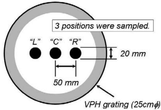
Fig. 3. Schematic view of the sampled positions on the VPH grating (referred to as “L”, “C”, and “R”). The region near the edge indicated in grey is occupied by the support structure of the grating mount and is not optically accessible.
