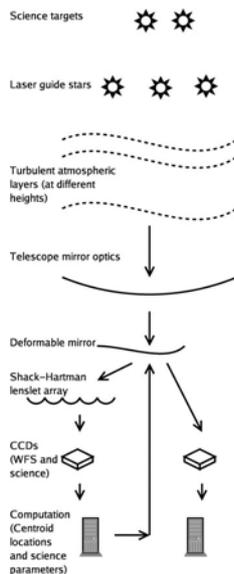
Fig. 5. Design of a GLAO system.
