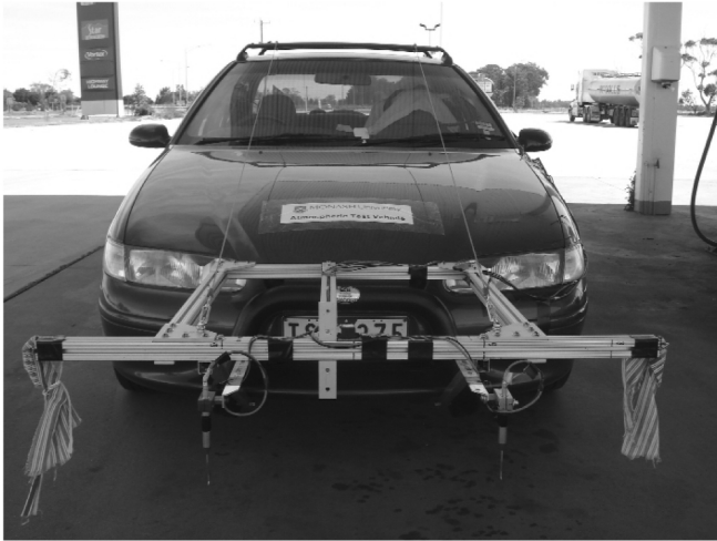
Figure 4. Probes mounted upstream of the vehicle for on-road measurement of flow conditions (from Wordley [11])
