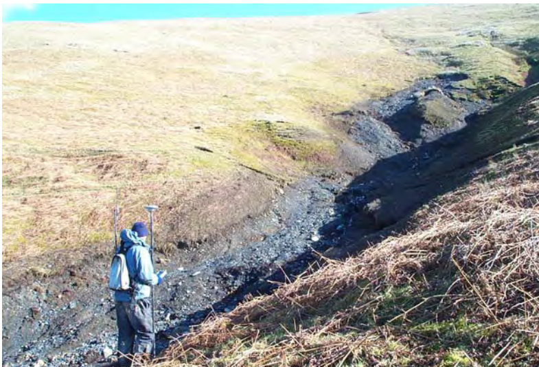
Figure 4. Cockup landslide runout channel (NY 253 313, 350 masl). Field survey of landslide extent using differential GPS.
