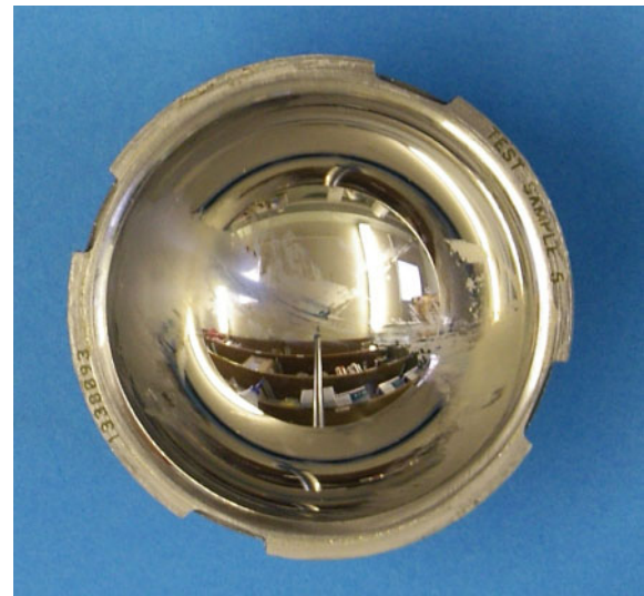
Fig. 4 Digital image of the deposit left on the Co-Cr-Mo alloy cup after 0.5 \times 10^6 cycles of wear testing in a standard walking-cycle simulator
