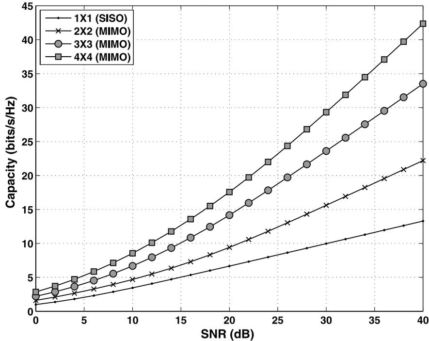
**Figure 7.** Estimates of channel capacity for various MIMO configurations corresponding to a 1-min data file measured at 1602 UT on 2 November 2007 and evaluated for different signal-to-noise ratios (between 0 and 40 dB).
