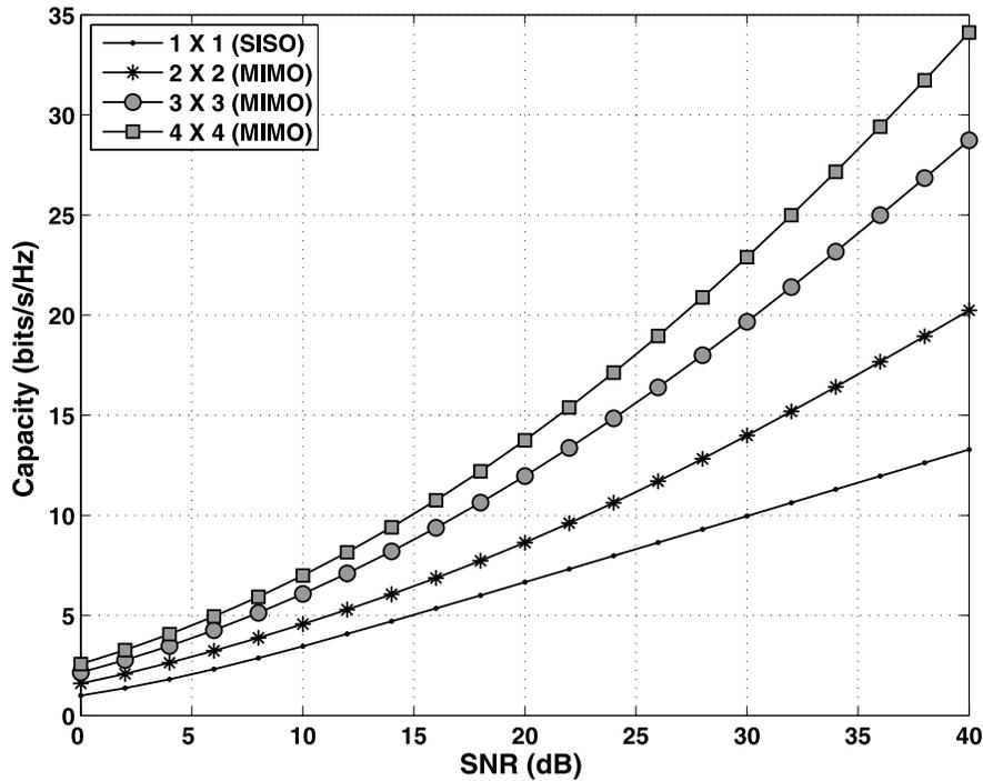
**Figure 11.** Plots of the average channel capacity for various MIMO configurations corresponding to data from a measurement campaign conducted on 3 September 2008 (79 1-min data files were analyzed) and evaluated for different signal-to-noise ratios (between 0 and 40 dB).
