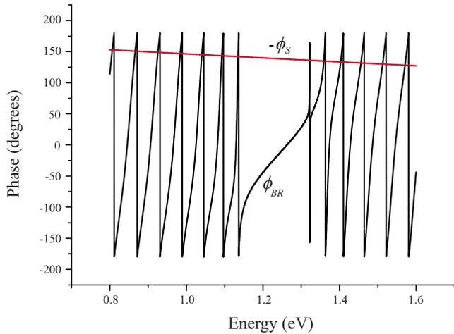
FIG. 2. (Color online) The phases  $\phi_{BR}$  and  $-\phi_S$  as a function of the energy of the incident light at an incident angle of  $\theta=45^\circ$  within the substrate. The crossing points indicate the energies at which “bound” photonic states are to be expected. (The vertical solid lines are an artifact of the plotting routine: at these points the phase shifts discontinuously from +ve to -ve values and hence these sections do not define crossing points.)
