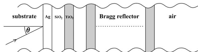
FIG. 1. The basic structure employed in most of the calculations, consisting of a left-hand substrate (SiO<sub>2</sub> in this case) with a thin silver (Ag) overlayer and a 40-layer SiO<sub>2</sub>/TiO<sub>2</sub> BR (20 layer pairs) on top. For the reflection coefficient calculations light is incident at an angle  $\theta$  from the left.
