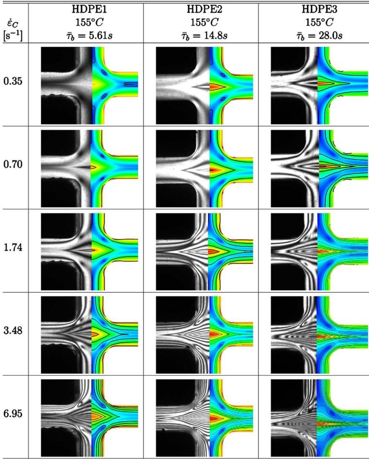
**FIG. 9.** Comparison between the experimentally observed flow-induced stress birefringence patterns for the HDPE series at different strain-rates with computed values of the principal stress difference shown with a contour interval of 22 kPa for all materials.
