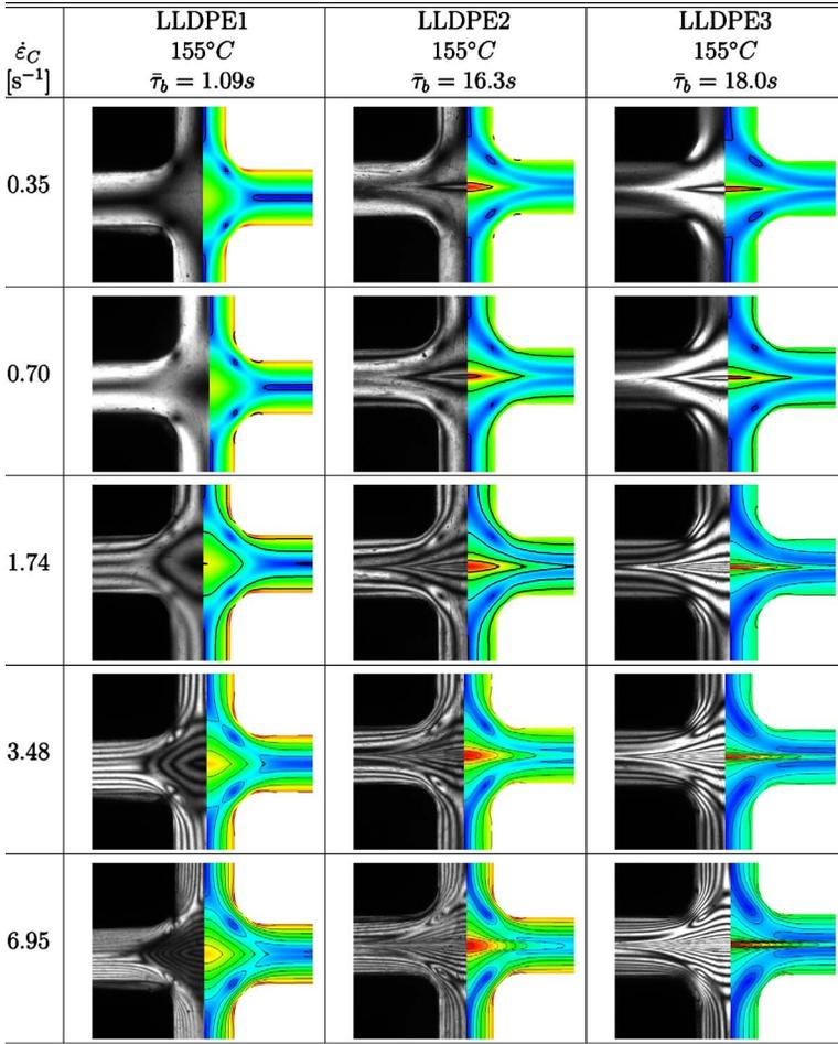
**FIG. 10.** Comparison between the experimentally observed flow-induced stress birefringence patterns for the LLDPE series at different strain-rates with computed values of the principal stress difference shown with a contour interval of 40 kPa for all materials.
