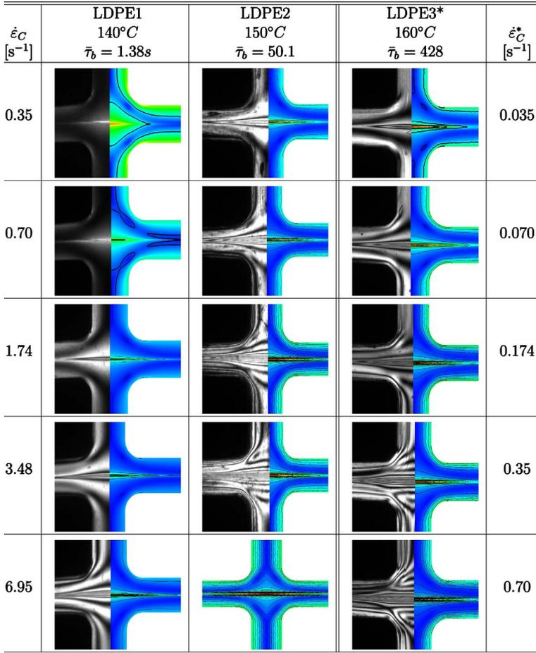
**FIG. 11.** Comparison between the experimentally observed flow-induced stress birefringence patterns for the LDPE materials at different strain-rates with computed values of the principal stress difference shown with using the same optical constant of 24.5 kPa for the three slowest flow-rates, and for clarity 49 kPa for the two fastest flow-rates. Note, for LDPE3 that the strain-rates are a factor 10 lower than for LDPE1 and LDPE2.
