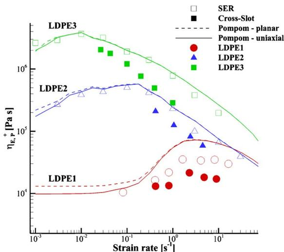
**FIG. 16.** Elongational viscosity  $\eta_E$  as a function of strain rate from uniaxial (open symbols) and cross-slot experiments (closed symbols) and together with the multimode Pom-pom predictions for the uniaxial (solid lines) and planar (dashed lines) extensional viscosity for the LDPE series.
