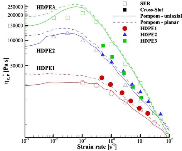
FIG. 14. Elongational viscosity  $\eta_E$  as a function of strain rate from uniaxial (open symbols) and cross-slot experiments (closed symbols) and together with the multimode Pompon predictions for the uniaxial (solid lines) and planar (dashed lines) extensional viscosity for the branched HDPE series.
