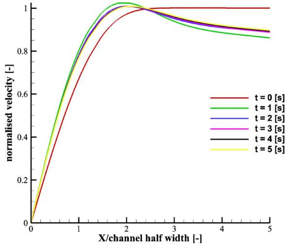
**FIG. 6.** A comparison of the velocity profile along the downstream symmetry line for the simulated HDPE3 Pompop spectrum as a function of time. Near the stagnation point the velocity increases where the Pompop modes are fully stretched leading to an overshoot in the velocity downstream.
