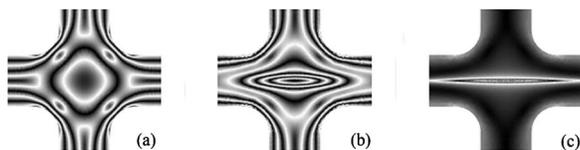
**FIG. 4.** Qualitative comparison of the predicted shape of the PSD for different flow Weissenberg number regimes for a single Pom-pom mode (with a solvent mode weighted at 10%): (a) slow flow, (b) orientating but non-stretching flow, and (c) stretching flow.
