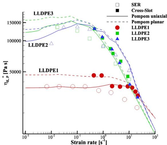
FIG. 15. Elongational viscosity  $\eta_E$  as a function of strain rate from uniaxial (open symbols) and cross-slot experiments (closed symbols) and together with the multimode Pompon predictions for the uniaxial (solid lines) and planar (dashed lines) extensional viscosity for the LLDPE series.
