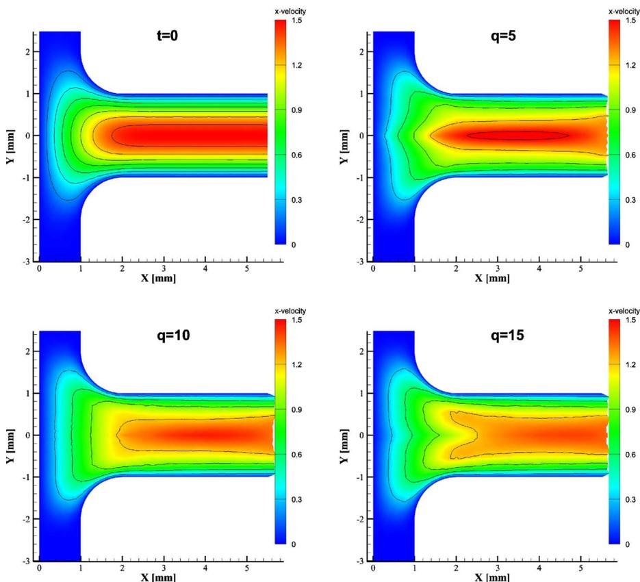
**FIG. 5.** Contour plots of the  $x$  velocity component in the right hand part of the cross-slot: (a) the initial Stokes solution, (b)  $q=5$ , the velocity near the stagnation point speeds up; (c)  $q=10$ ; d) for large values of  $q=15$  the large stretch gradient slows the flow down. Parameters chosen were  $G=0.9$ ,  $\tau_b=10$ , and  $\tau_s=10$  with varying  $q$ , this gives an initial Weissenberg number of 10 for both stretch and orientation
