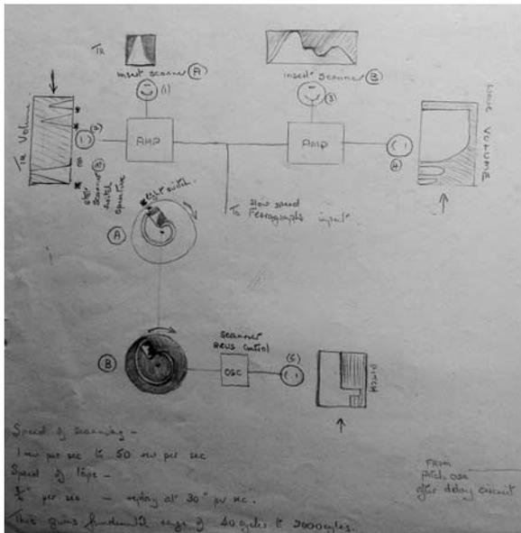
**Figure 3.** The proposed design for a disk-based waveform scanner, 1957
