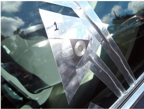
**Figure 7. Detailed view of surface microphone attachment**
