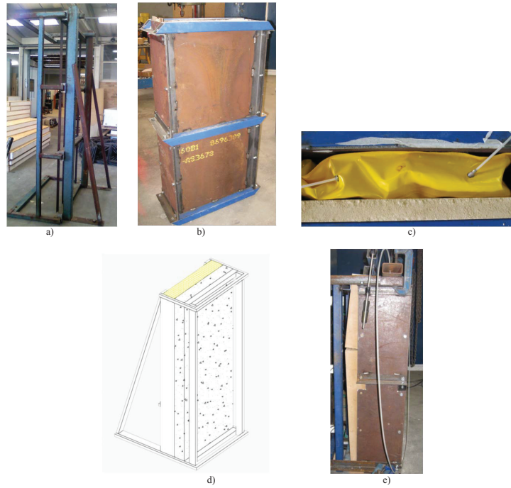
Fig. 3 Experimental setup. a): steel frame constraining the rammed earth wall; b): ramming formwork; c): top view of the not fully inflated airbag; d): complete experimental scheme; top of e): clamped steel bars generating the pre-load P .
