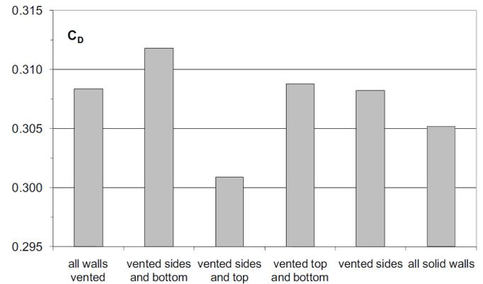
Figure 6. Effect of venting individual cavity walls.
