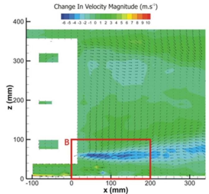
Figure 13. Change in vector field on Centreline when underside slots are closed (Ventilated Cavity 90mm deep)
