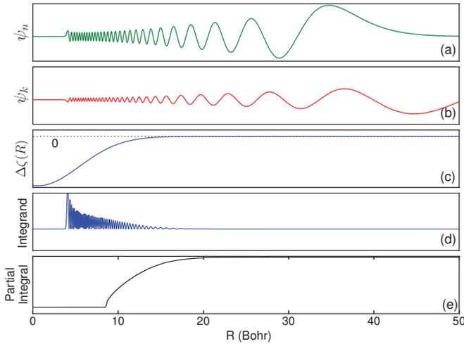
FIG. 5. (Color online) The functions contributing to the integral  $I_{nk}$  of Eq. (18) for CsYb. (a) Wave function for the  $n = -4$  bound state,  $\psi_{n=-4}(R)$ , which is the shallowest bound state for which crossings can exist. (b) Wave function for the low-energy continuum state,  $\psi_k(R)$ . (c)  $\Delta\zeta_a(R)$ . (d) The integrand of the matrix element  $\psi_n\psi_k\Delta\zeta$ . (e) The partial integral  $\int_0^R \psi_n(R')\psi_k(R')\Delta\zeta(R')dR'$ .
