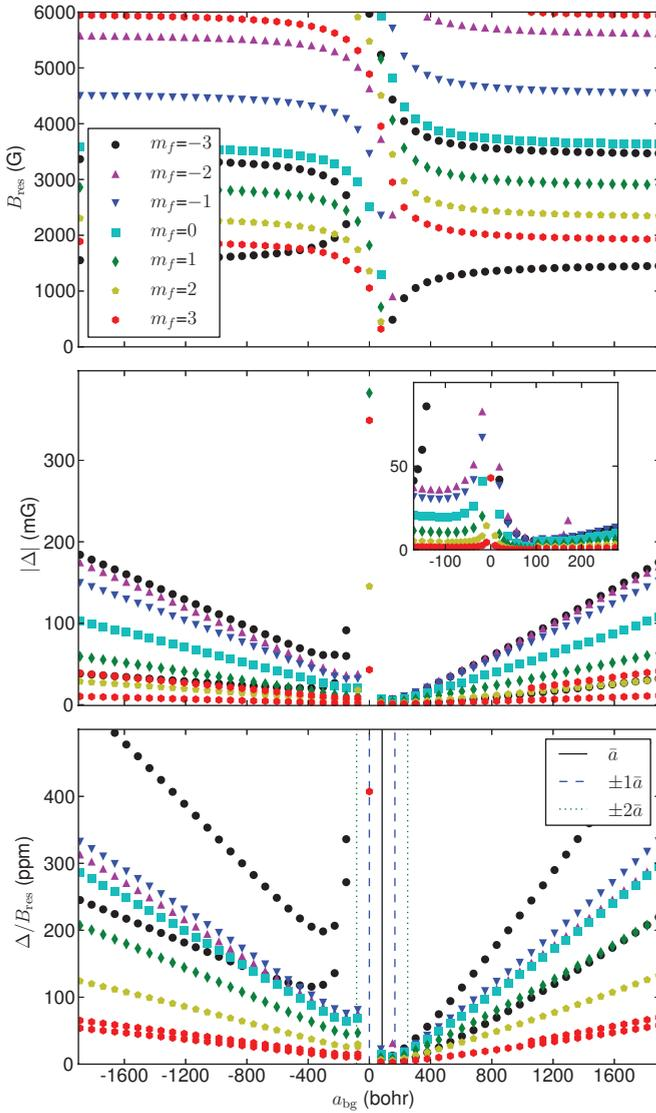
FIG. 8. (Color online) Resonance positions and widths for  $^{133}\text{Cs}^{174}\text{Yb}$ , obtained from coupled-channel calculations, as a function of the background scattering length  $a_{\text{bg}}$ . Top panel: Resonance position  $B_{\text{res}}$ . Center panel: Width  $|\Delta|$ , with an inset showing an expanded view for values of  $a_{\text{bg}}$  near the mean scattering length  $\bar{a}$ . Bottom panel:  $\Delta/B_{\text{res}}$  in parts per million.
