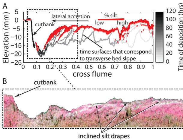
**Figure 4:** Cross-sections of point-bar deposits from experiment (case 8). a) Synthetic slice through experimental point-bar deposit, showing cohesive sediment layers and time of deposition. b) Sediment peel from same location as shown in (a).
