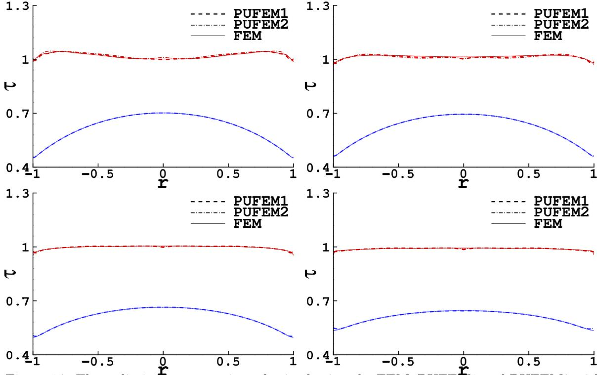
Figure 16: The radiative energy ratio  $\tau$  obtained using the FEM, PUFEM1 and PUFEM2 with  $\varepsilon = 1$  (blue lines) and  $\varepsilon = 0.1$  (red lines) for the conduction-radiation in a disc enclosure after 5 time steps (top left), 10 time steps (top right), 50 time steps (bottom left) and 200 time steps (bottom right).
