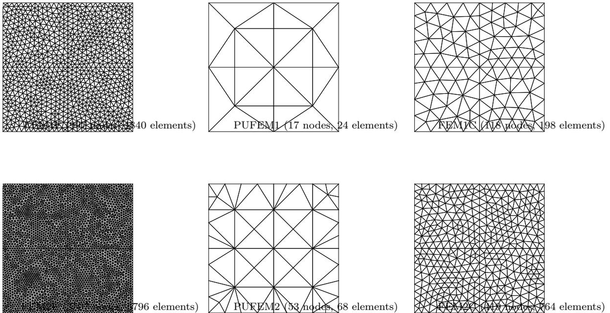
Figure 2: Coarse meshes (first row) and fine meshes (second row) used for the comparison between the FEM and the PUFEM for the conduction-radiation in a square enclosure.
