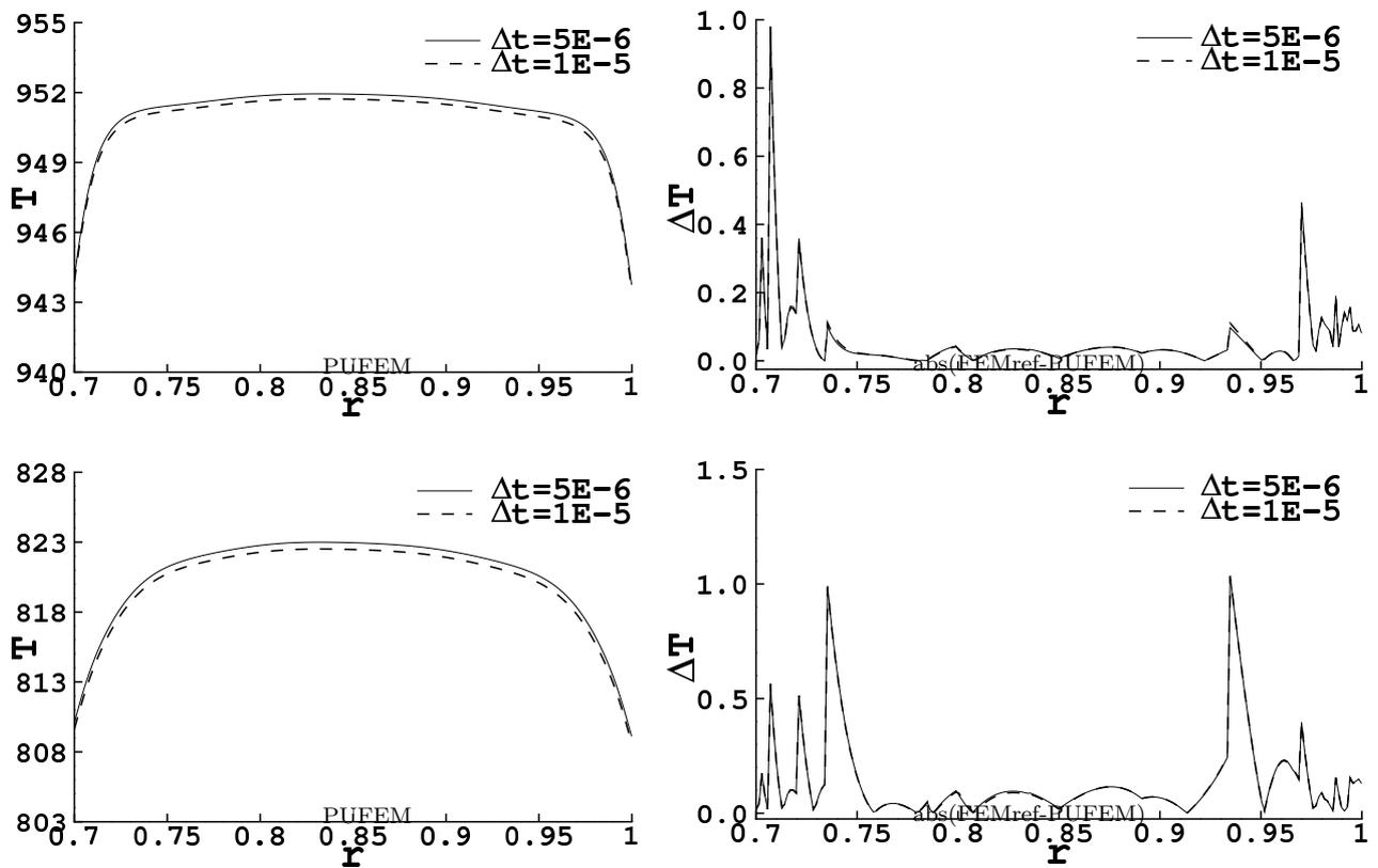
Figure 10: Radial cross-section of the temperature distribution (left column) and its associated differences (right column) using two different time steps for the conduction-radiation in a ring enclosure using  $\varepsilon = 1$ . The final time is  $10^{-4}$  (first row) and  $5 \times 10^{-4}$  (second row).
