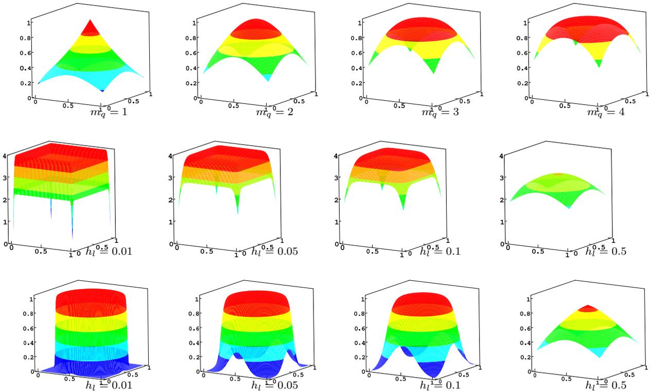
Figure 1: Illustration for different orders of enrichment functions of the Gaussian (first row) and the hyperbolic tangent on four edges of a square (second row) and on a circle (third row).
