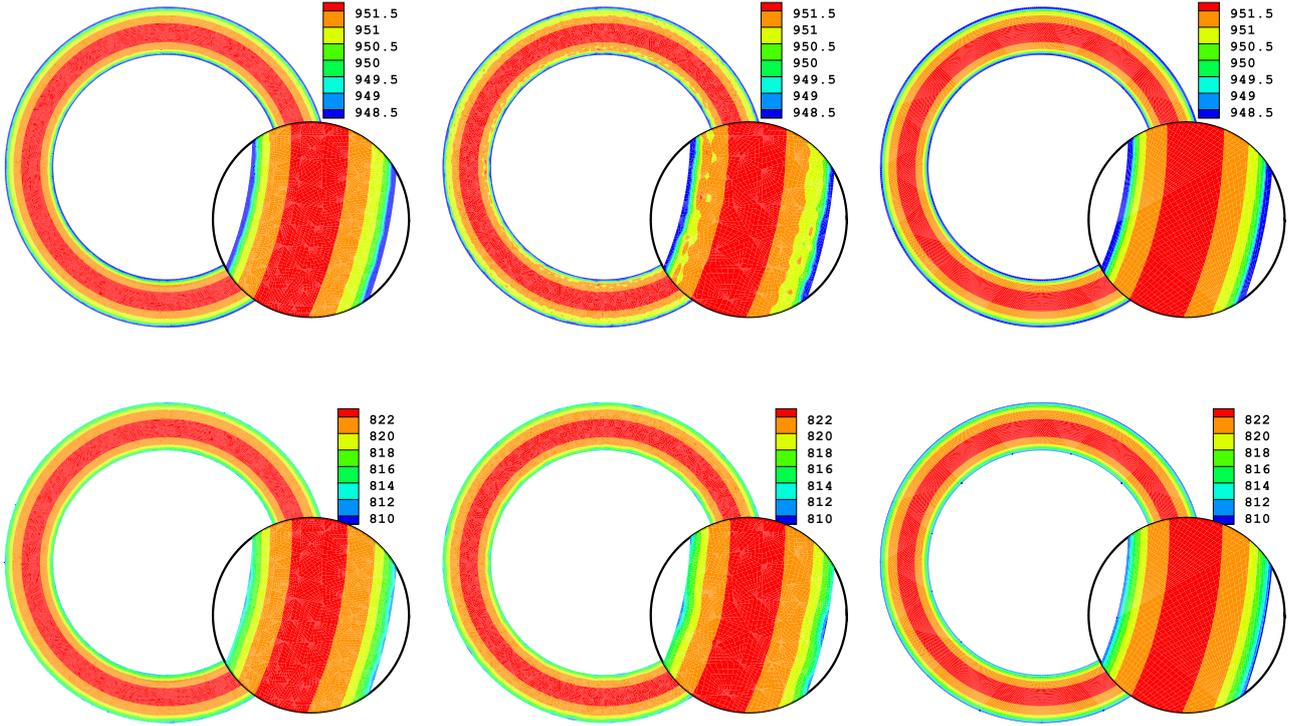
Figure 7: Temperature distribution obtained using FEMf (first column), FEMc (second column) and PUFEM (third column) after 10 time steps (first row) and after 50 time steps (second row) for the conduction-radiation in a ring enclosure using  $\varepsilon = 1$ . A zooming is also shown in these results.
