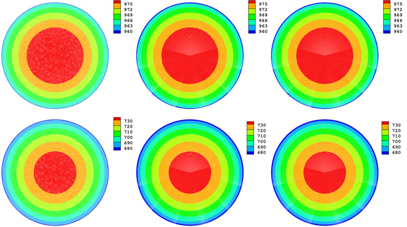
Figure 12: Temperature distribution obtained using FEM (first column), PUFEM1 (second column) and PUFEM2 (third column) after 10 time steps (first row) and after 200 time steps (second row) for the conduction-radiation in a disc enclosure using  $\varepsilon = 1$ .
