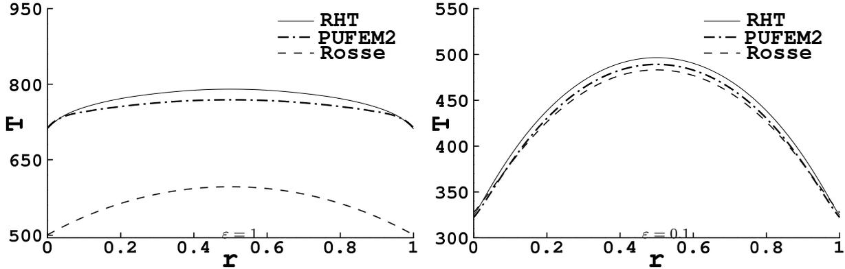
Figure 5: Cross section of the temperature at main diagonal in the enclosure obtained using the full RHT, Rosseland and PUFEM models for  $\varepsilon = 1$  (left plot) and  $\varepsilon = 0.1$  (right plot) after 100 time steps for the conduction-radiation in a square enclosure.
