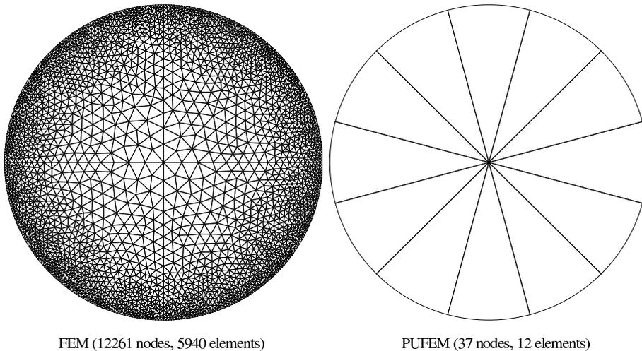
Figure 11: The unstructured meshes used for the problem of conduction-radiation in a disc enclosure.
