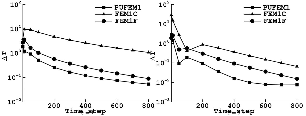
Figure 3: Time evolution of the temperature differences at the corner ( $x = 0, y = 0$ ) on the coarse meshes for  $\varepsilon = 1$  (left plot) and  $\varepsilon = 0.1$  (right plot) for the conduction-radiation in a square enclosure.
